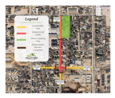
These closures are taking place so that concrete along both sides of 4<sup>th</sup> Avenue South can be poured, dried, and cured safely and efficiently. Once this has been done, the remaining driveway restoration and asphalt preparation can begin.
